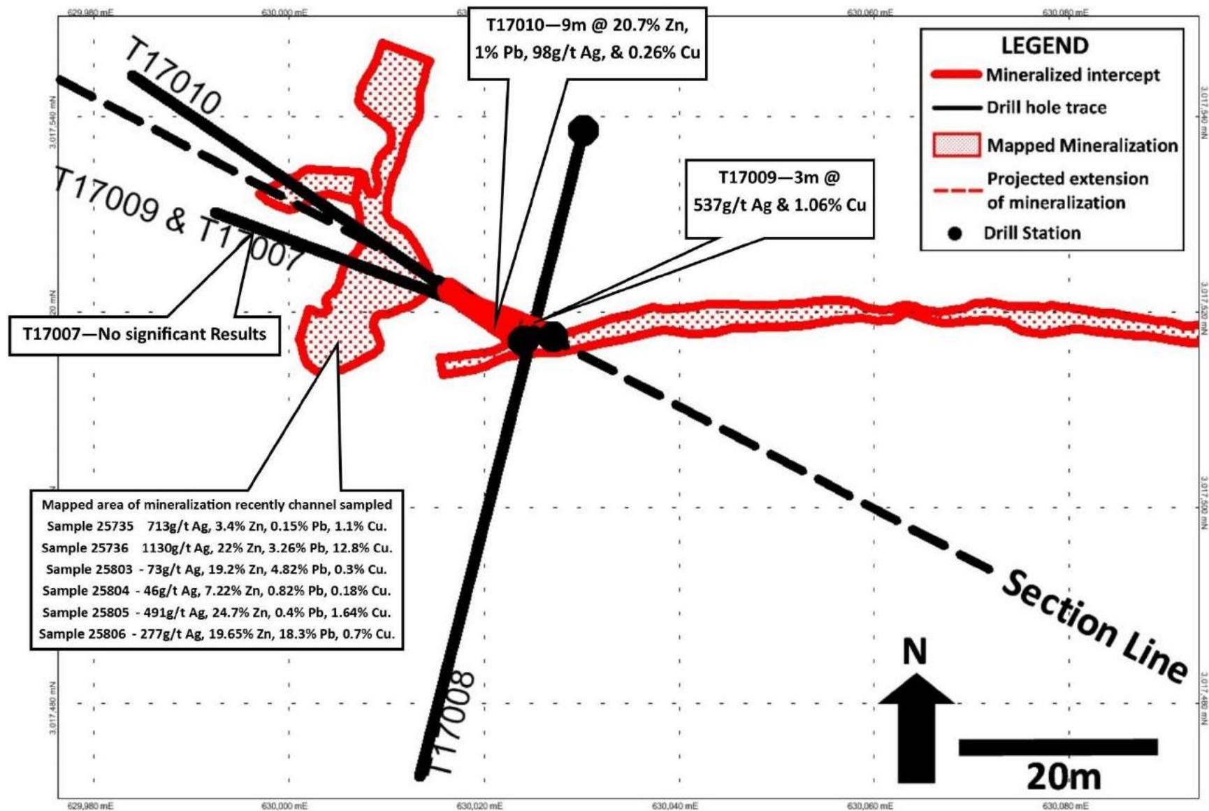
Figure 3. Location map of the channel samples in relation to the surveyed underground workings and mapped zones of mineralization. Also shown are the planned sites for the drill program currently underway.
